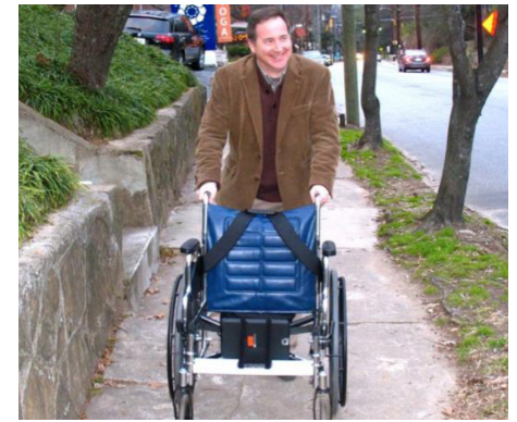
Figure 1.1: The Sidewalk Sentry data collection system utilized a tablet which recorded rolling video along with tilt and vibration information.
